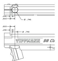
2. Use the CenterFeed as a template to centerpunch the sidehole.
